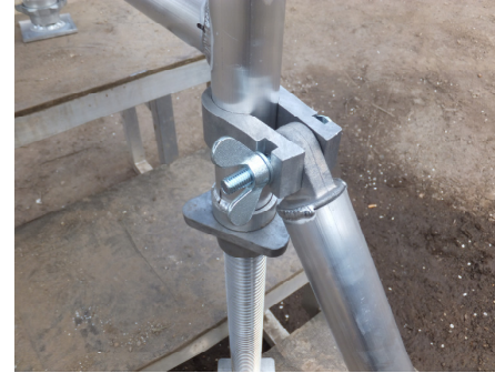
3. POSITION PODIUM, ADJUST LEGS TO LEVEL UNIT AND FIX STABILISERS. TIGHTEN WING NUTS FINGER TIGHT.
